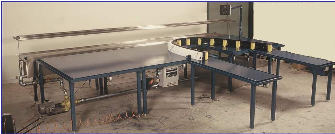
The **VBS 3000** is designed to give manufacturers the ability to bend vinyl extrusions and create any type or style of arched window. The versatile **VBS 3000** can accommodate round arches, extended arches with sides, segmented arches and elliptical shapes and, you can bend radii as small as 12 inches.
