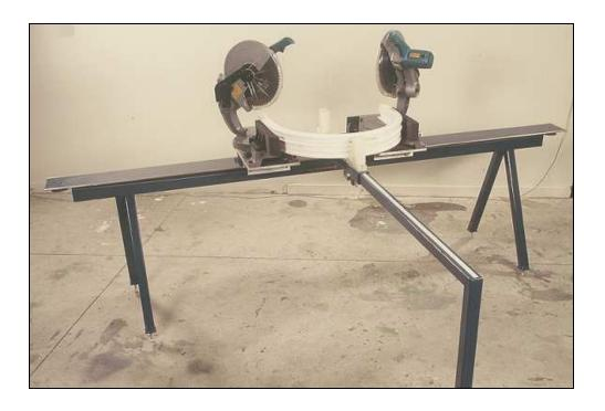
The RTS 1000 compliments the VBS 3000 and cuts both round tops and straight edges in one simple set-up. Coupled with Opticut's Special Shapes Software, material requirements and angles are automatically calculated for a perfect fit every time.
