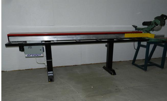
With the **Opti-Stop Max** you can automate a wide variety of manufacturing functions and eliminate cutting errors, adding to the life of your cutting and boring tools. No need to run network cables to the shop floor, nor do you need to tether the controller to the machine. WiFi and Bluetooth technology tie the system together, wirelessly
