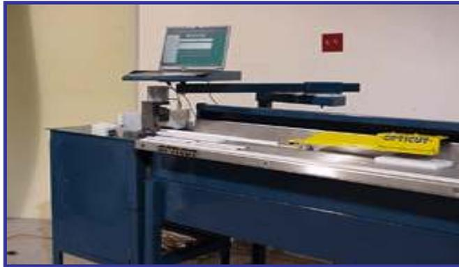
The **Auto WinGrid 1600** is a versatile automated saw for all window grill styles, spacer bars and screen frames. The machine reads from pre-programmed, optimized cutting lists and performs cuts, notches, and punches with material being advanced by an automated pusher and can be used as an automated length stop.
