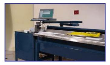
The Auto WinGrid 1600 is a versatile automated saw for all window grill styles, spacer bars and screen frames.
